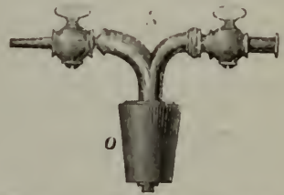
FIG. 78. The Stopper and Cocks supplied with Apparatus No. 2.
